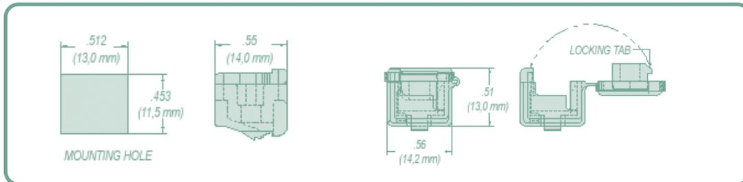
Assembly friendly! Independent of insertion into the panel, Lockit Strain Reliefs self-lock on the cable. They may be pre-assembled offline for final assembly at a later time or remote location for lower installed cost. Perfect for jobs in the field.
