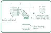
All the same functions as the straight connectors but offer more flexibility. Complete connector is reusable. Smooth internal surfaces for easier wire installation.
